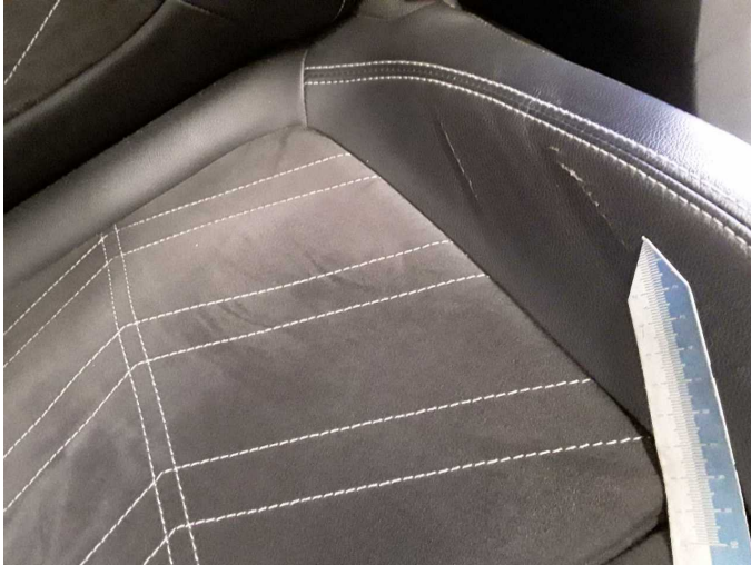
Damage 1: Seat - front: Seat cover - left side - Porous / cracked - Replace
