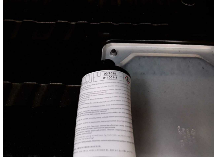
Damage 1: Equipment: Tirefit filler - Expired - Replace
