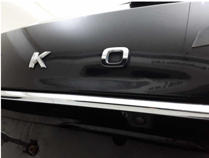
Damage 6: Boot lid / rear door: Boot lid glazed - dent(s) - Repair and paint
