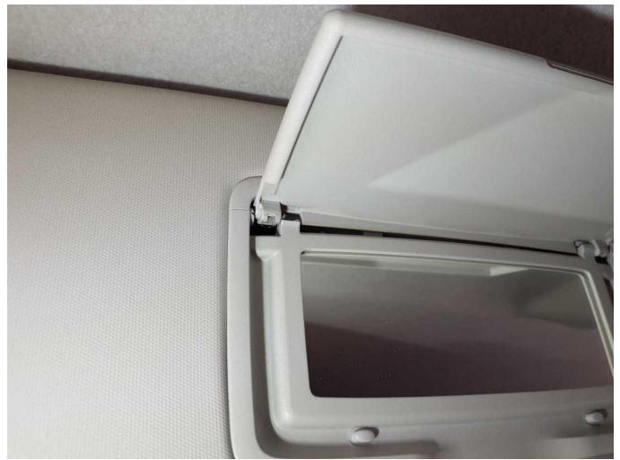
Damage 1: Interior: Sun visor - left side - Broken / torn - Replace
