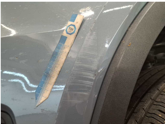
Damage 5: Front bumper: Front bumper - Scratched - Paint
