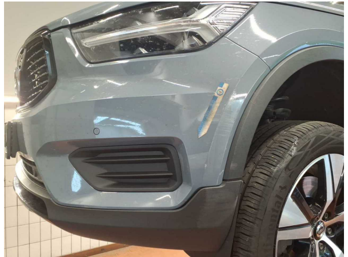
Damage 5: Front bumper: Front bumper - Scratched - Paint
