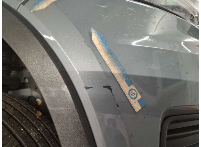
Damage 5: Front bumper: Front bumper - Scratched - Paint
