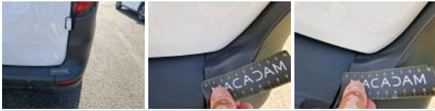
Bumper R, Hole, Repair and paint (complete)
