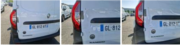
Boot door panel RL, Dent(s) and scratch(es), Repair and paint (complete)
