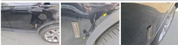
Wing trim RL, Scratch(es), Replace
