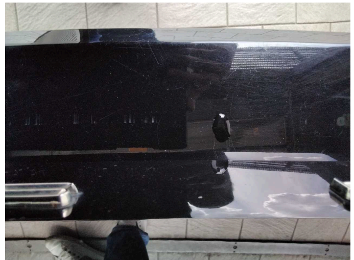
Damage 10: Rear bumper: Rear bumper - Scratch(es) - Paint
