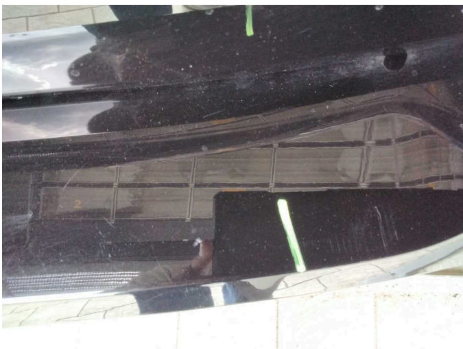
Damage 10: Rear bumper: Rear bumper - Scratch(es) - Paint
