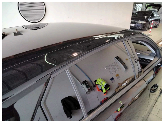
Damage 9: Roof: Roof rail - right side - Dent / paintcoat damage - Repair and paint
