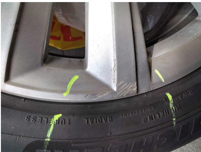
Damage 8: 2nd wheel set: 1 alloy rim - Scratch(es) - Loss in value
