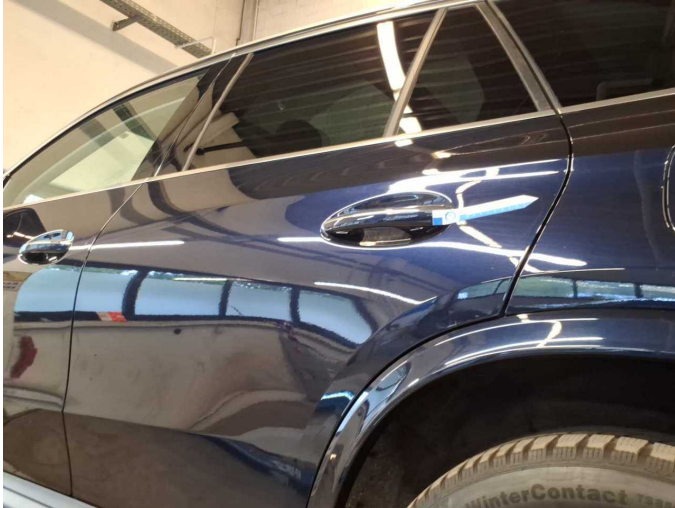
Wear and tear 1: Door - rear left side: Door edge - Scratched - No deduction
