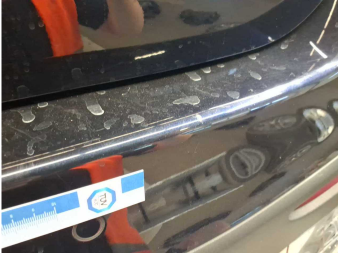
Damage 7: Rear bumper: Rear bumper - Scratched - Paint
