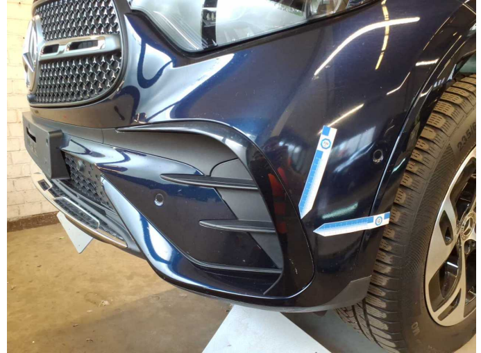
Damage 4: Front bumper: Cover bumper - front - Deformed - Replace
