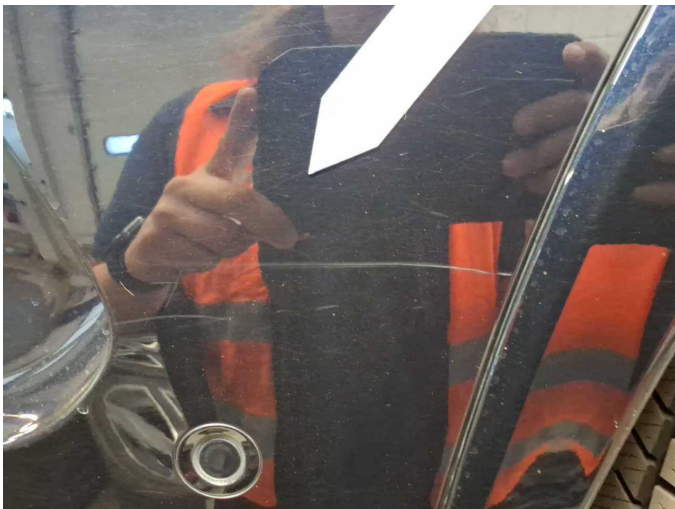
Damage 7: Rear bumper: Rear bumper - Scratched - Paint
