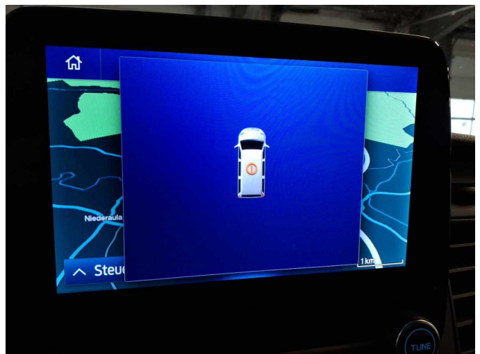
Damage 4: Electronic systems: Parking assistance - Functional / admissibility - Perform diagnosis
