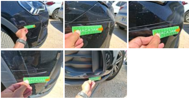
Bumper moulding F, Broken, Replace
