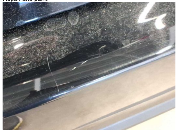
Damage #16: Rear bumper: Rear bumper - Scratch(es) - Repair and paint
