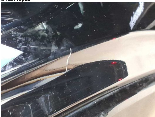
Damage #11: Side panel - rear right side: Sill - Scratch(es) - Smart repair
