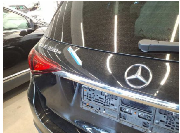
Damage #9: Boot lid / rear door: Boot lid - dent(s) - Smooth repair work
