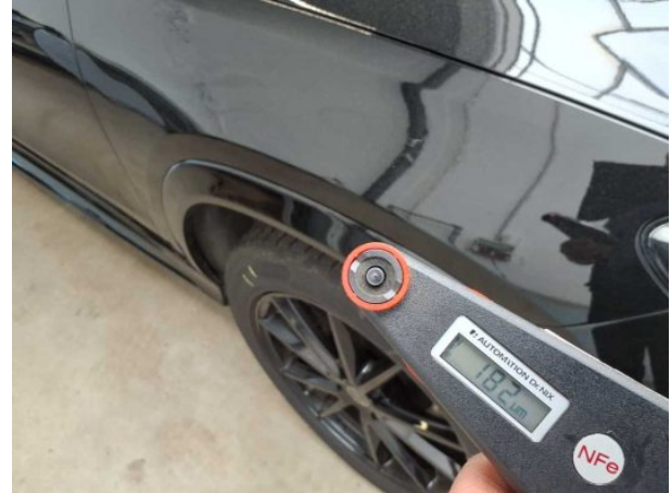
Repainting 1: Mudguard - right side
