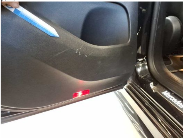
Damage #18: Trim / covers: Door trim - rear left side - Scratch(es) - Replace
