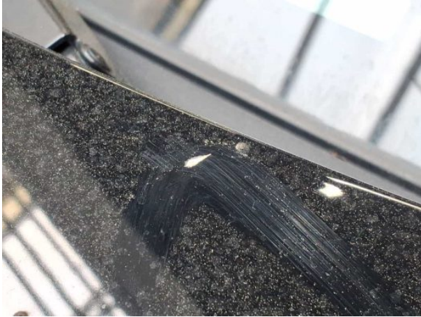
Damage #12: Bonnet: Bonnet - Scratch(es) - Smart repair
