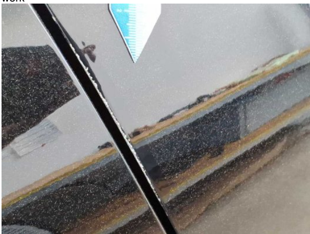
Damage #10: Door - rear right side: Door edge - Scratch(es) - Smart repair
