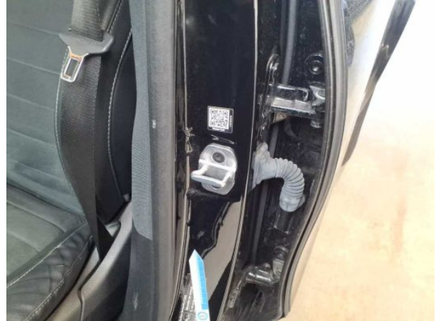
Damage #8: Body: B-pillar - left side - dent(s) - Smooth repair work
