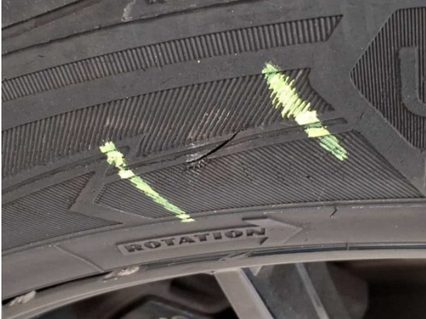
Damage #15: Wheel / tyres: Tyre - front right side - Broken / torn - Replace
