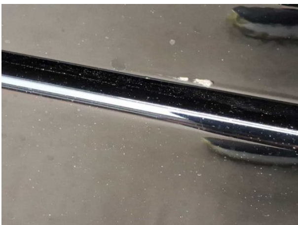
Damage #3: Door - rear right side: Door - Scratch(es) - Cover / polish
