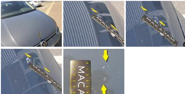
Wing RR, Dent(s), Repair and paint (complete)
