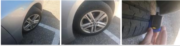
Tyre FL, Out of tolerance, Replace
