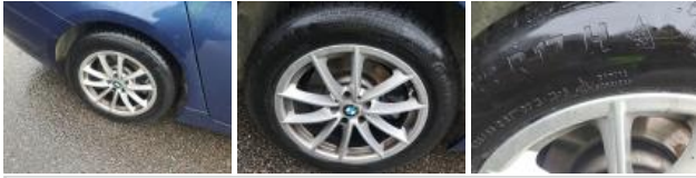
Tyre RL, Out of tolerance, Replace
