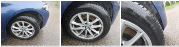
Tyre RR, Out of tolerance, Replace
