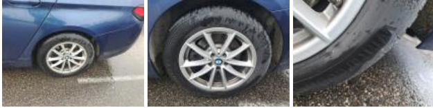
Tyre FL, Out of tolerance, Replace
