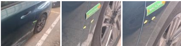
Wing RR, Dent(s), Repair and paint (complete)
