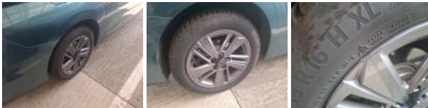
Tyre FR, Out of tolerance, Replace
