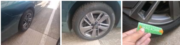
Tyre RR, Out of tolerance, Replace
