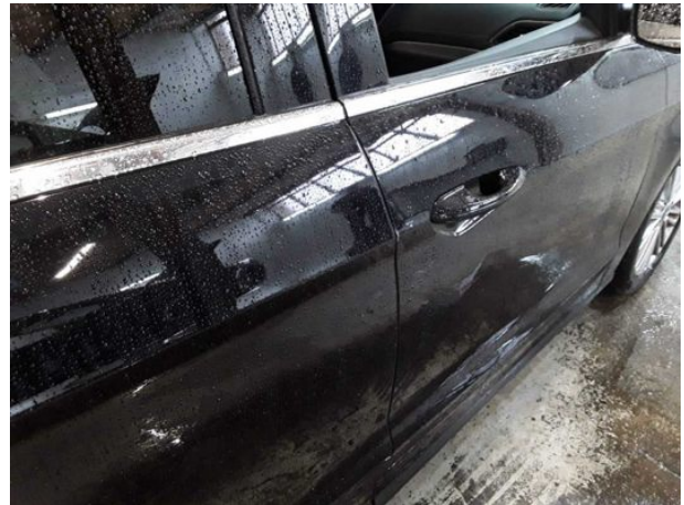
Damage #2: Door - rear right side: Door - Scratched - Smart repair
