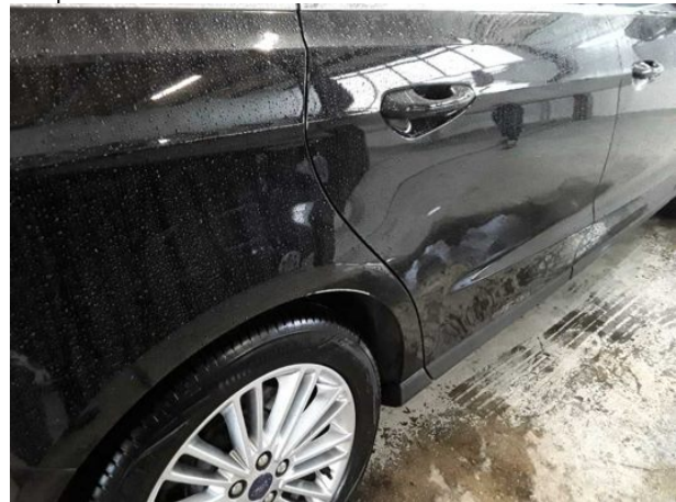
Damage #6: Side panel - rear right side: Side panel - Scratch... - Repair and paint
