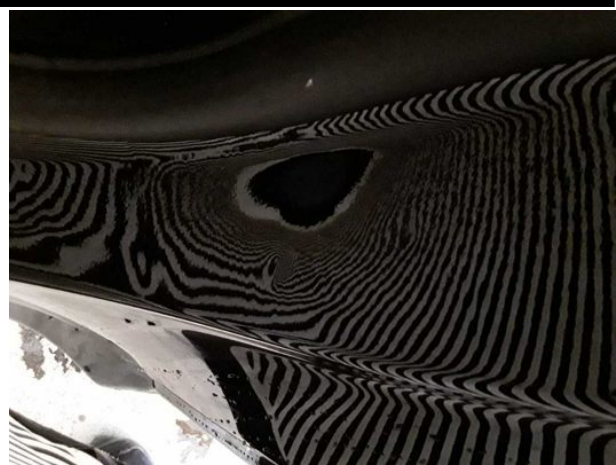
Damage #3: Side panel - rear left side: Sill - Dent / paintcoat damage - Repair and paint
