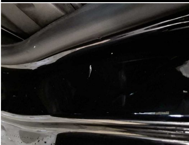
Damage #3: Side panel - rear left side: Sill - Dent / paintcoat damage - Repair and paint
