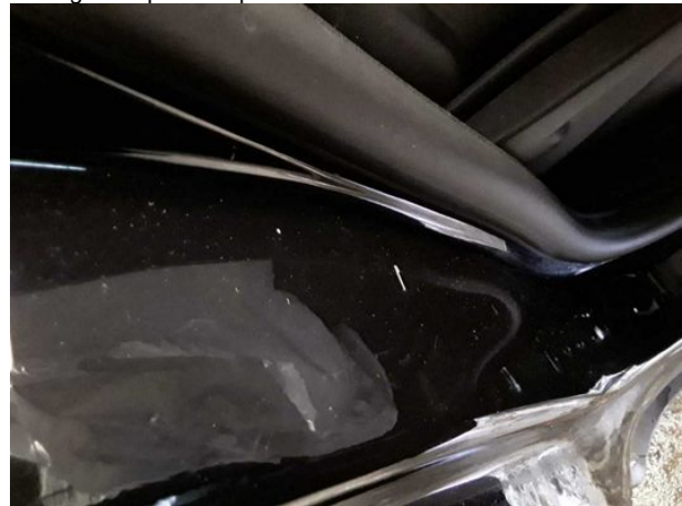
Damage #4: Side panel - rear right side: Sill - Dent / paintcoat damage - Repair and paint
