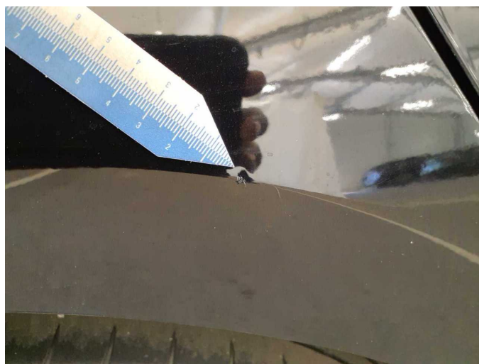
Damage 6: Side panel - rear right side: Side panel - Dent / paintcoat damage - Smart repair
