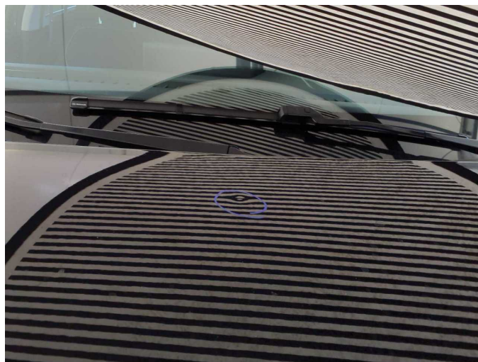
Damage 5: Bonnet: Bonnet - dent(s) - Smart repair
