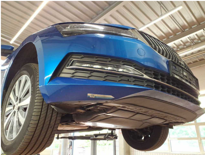
Damage 7: Front bumper: Front bumper - Scratched - Paint
