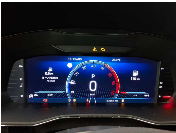
Damage 5: Instrument panel: Indicator light (Motor) - Electrical fault - Perform diagnosis
