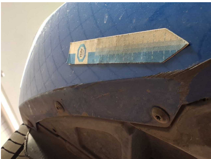
Damage 7: Front bumper: Front bumper - Scratched - Paint
