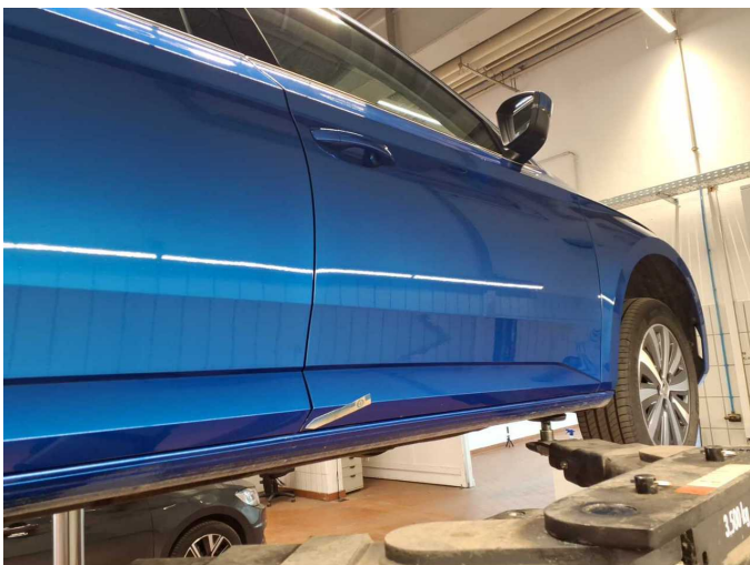
Damage 1: Door - front right side: Brightware - lower - Scratch(es) - Smart repair
