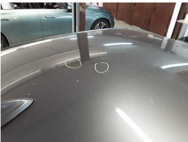
Damage #10: Roof: Roof - dent(s) - Smooth repair work
