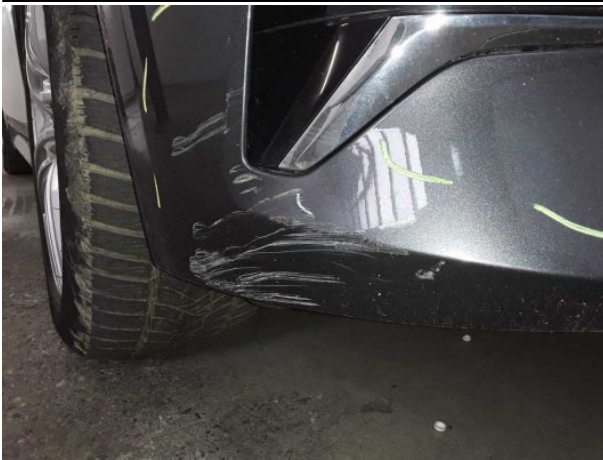
Damage #13: Front bumper: Front bumper - Scratched - Repair and paint
