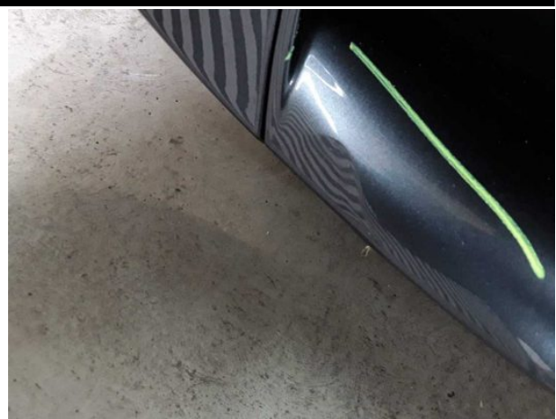
Damage #11: Front bumper: Spoiler - Deformed - Replace
