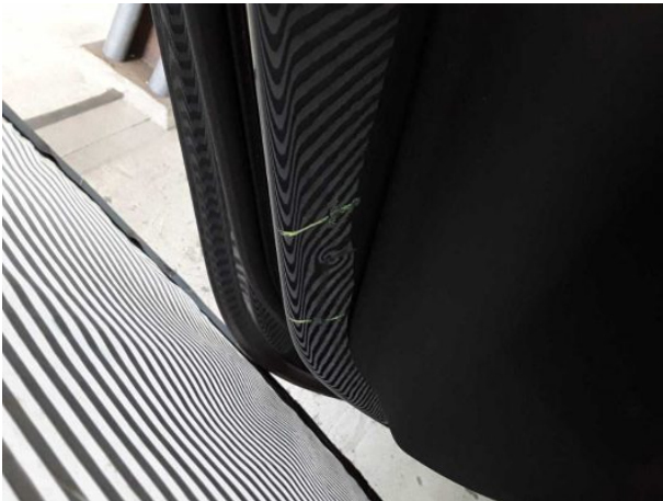
Damage #9: Door - rear left side: Door - Scratched - Smart repair
