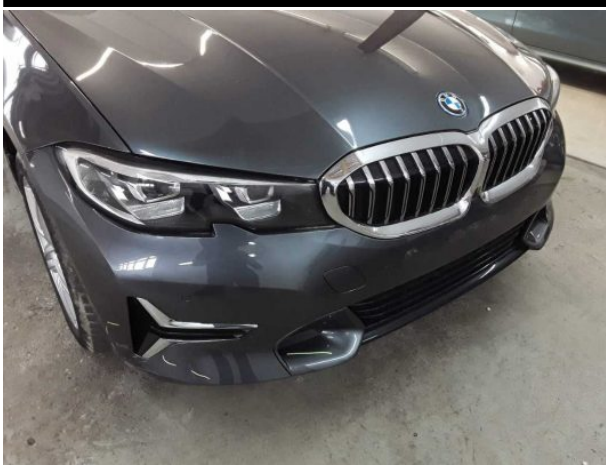
Damage #11: Front bumper: Spoiler - Deformed - Replace
