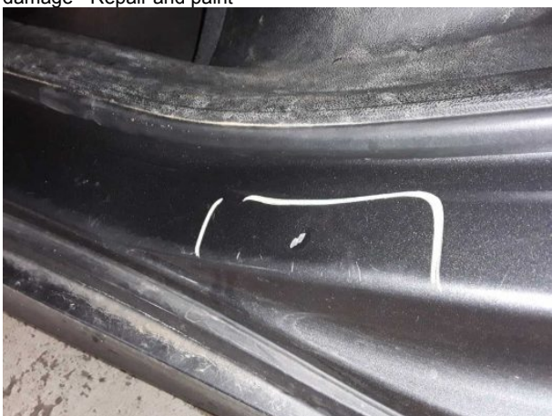
Damage #12: Side panel - rear left side: Sill - Dent / paintcoat damage - Repair and paint
