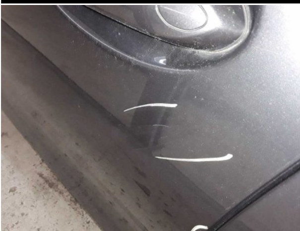
Damage #8: Door - front left side: Door - Scratched - Smart repair
