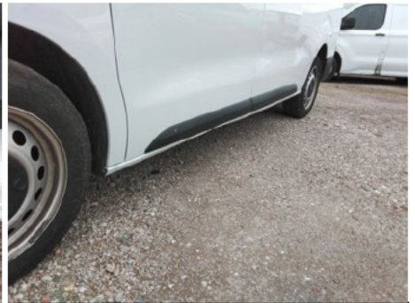
Schweller / Vorne Links / Delle
