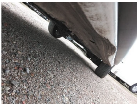
Schweller / Vorne Links / Delle
