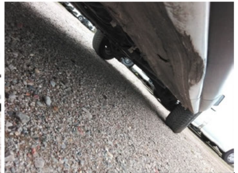
Schweller / Vorne Links / Delle
