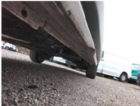
Schweller / Vorne Links / Delle
