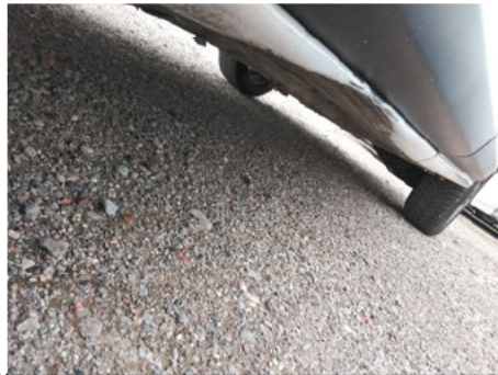
Schweller / Vorne Links / Delle
