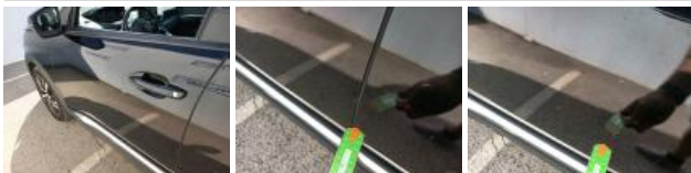
Wing FL, Scratch(es), Repair and paint (complete)
