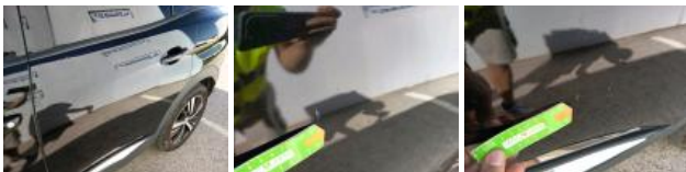
Door FL, Scratch(es), Repair and paint (complete)
