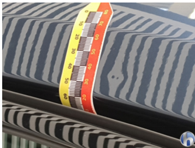
6. Dachrahmen - Links 1 Delle - Sanft Instandsetzen
