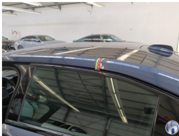
6. Dachrahmen - Links 1 Delle - Sanft Instandsetzen
