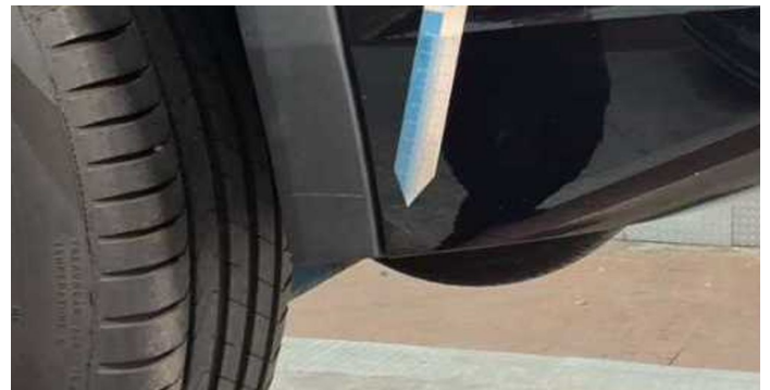
Damage 1: Side panel - rear left side: Wheel well extension - Scratch(es) - Smart repair
