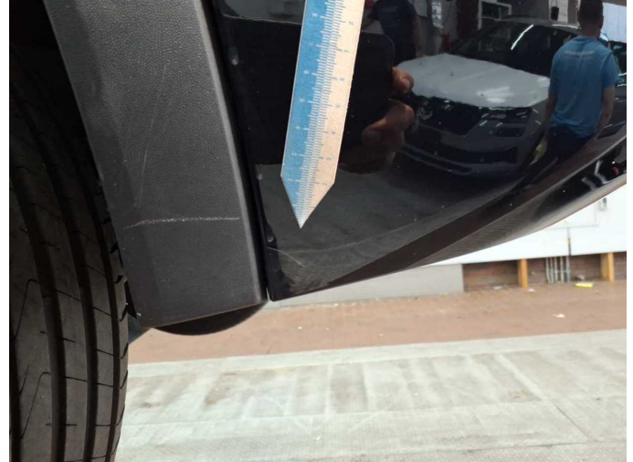
Damage 3: Rear bumper: Spoiler - Scratch(es) - Smart repair
