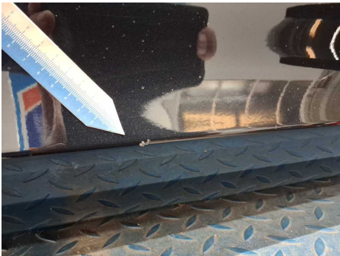
Damage 6: Door - front right side: Brightware - lower - Scratch(es) - Replace
