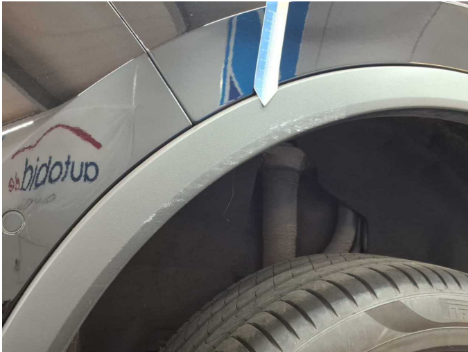
Damage 7: Side panel - rear right side: Wheel well extension - Paint defect - Replace
