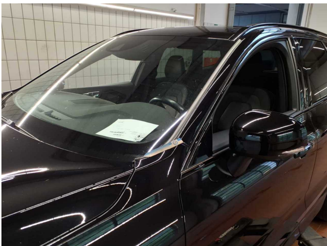
Damage 3: Front structure: Windscreen air deflector (Links) - Damage caused by marten / rodent - Replace
