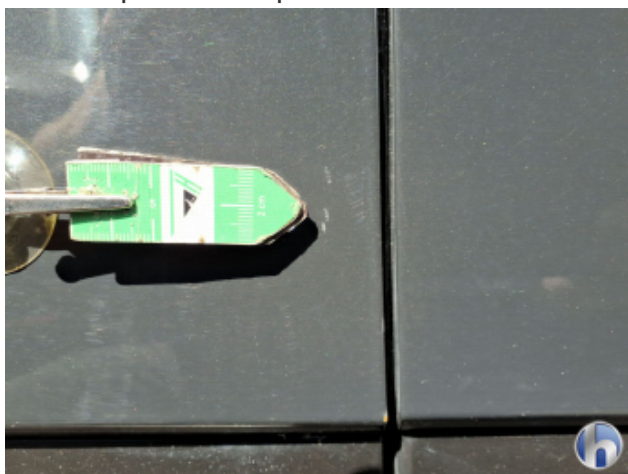
5. Tür Vorne - Links Kratzer - Smart Repair
