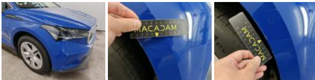
Bonnet, Bad repair, Repair and paint (complete)
