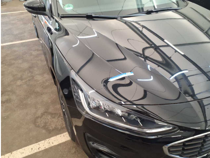
Damage 1: Bonnet: Bonnet (Ätzungen, Vogelkot) - Paint defect - Smart repair
