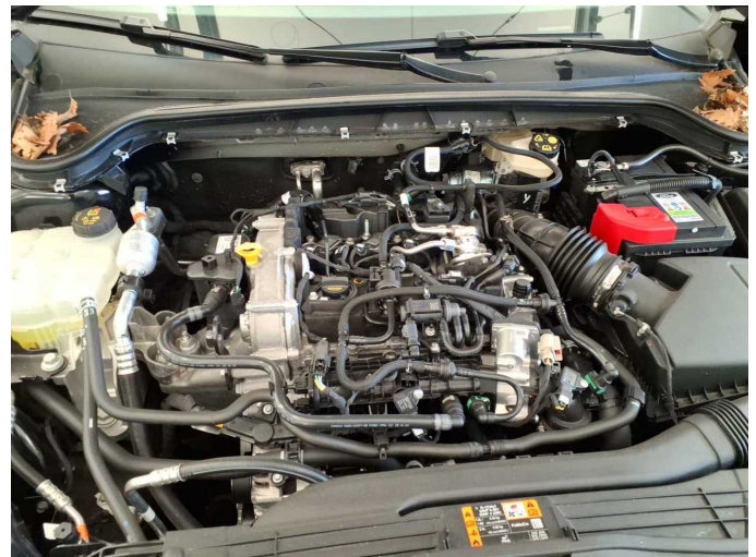
Missing part 1: Engine: Engine cover - Missing - Replace
