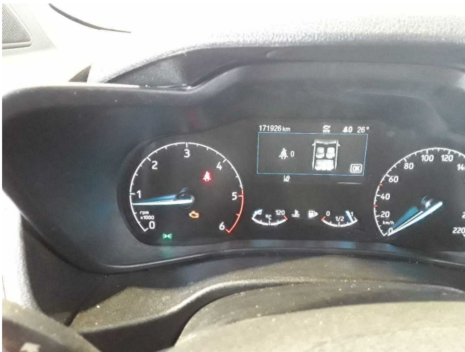
Damage 5: Instrument panel: Indicator light (Motorkontrolle) - on - Perform diagnosis
