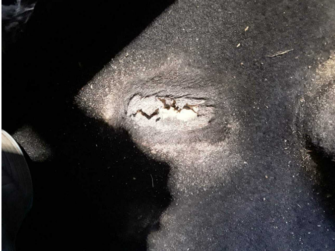
Damage 10: Trim / covers: Carpet - front left side - Worn - Replace
