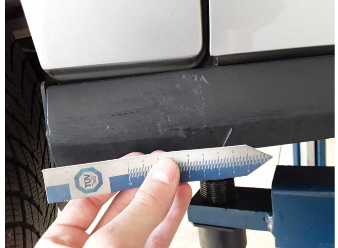
Damage 4: Sill - right side: Trim - Scratch(es) - Replace
