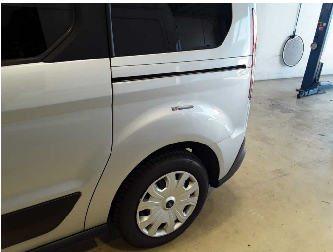
Damage 9: Side panel - rear left side: Side panel (Spachtel eingefallen) - Unprofessionally repaired - Paint
