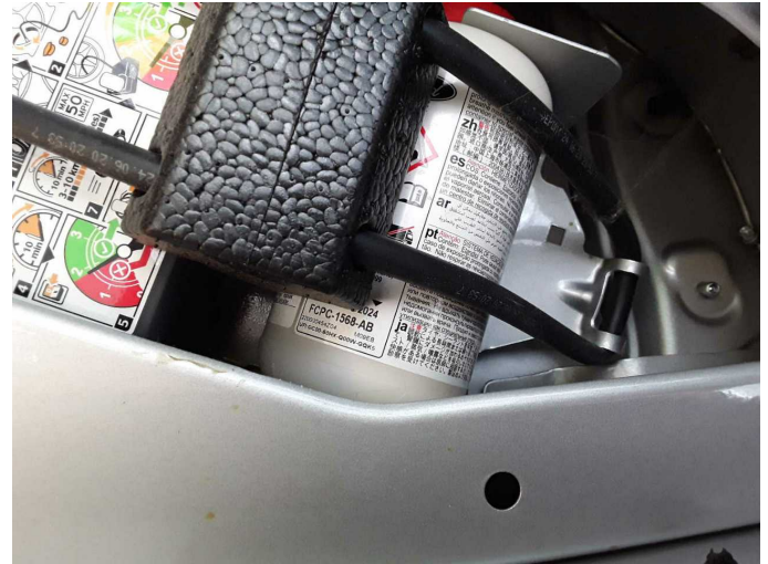
Damage 1: Equipment: Tirefit filler - Expired - Replace
