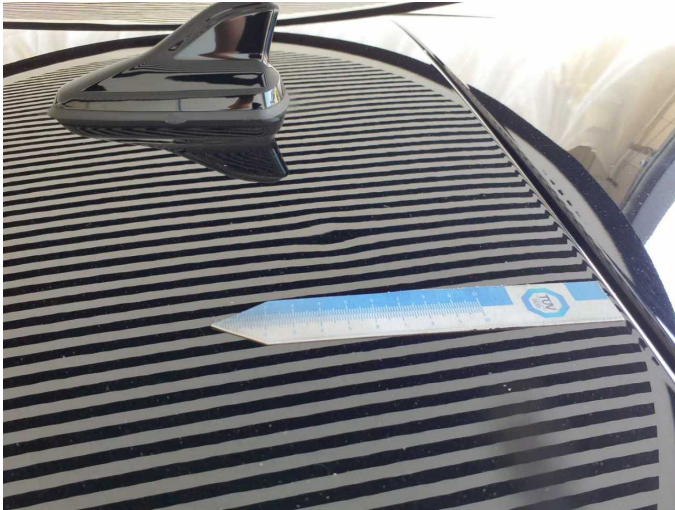
Damage 1: Roof: Roof - dent(s) - Smooth repair work
