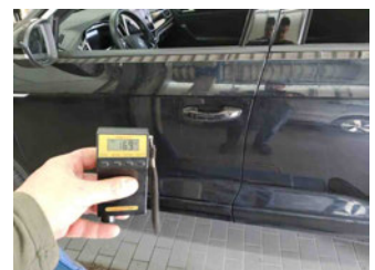
Paint thickness Door FL
