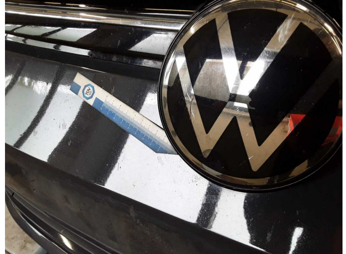
Damage 3: Bonnet: Emblem - Damaged - Replace
