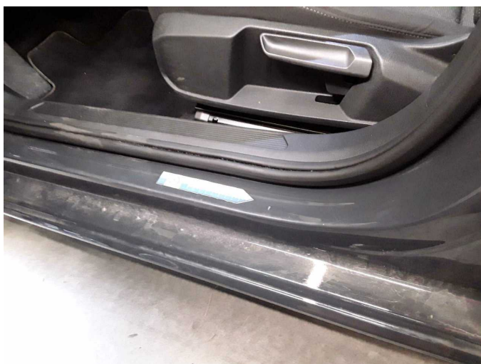
Damage 2: Sill - left side: Sill - Dent / paintcoat damage - Smart repair
