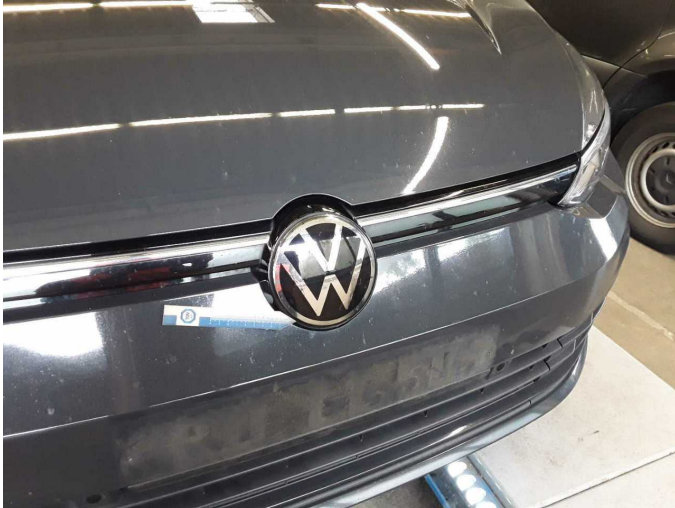
Damage 3: Bonnet: Emblem - Damaged - Replace
