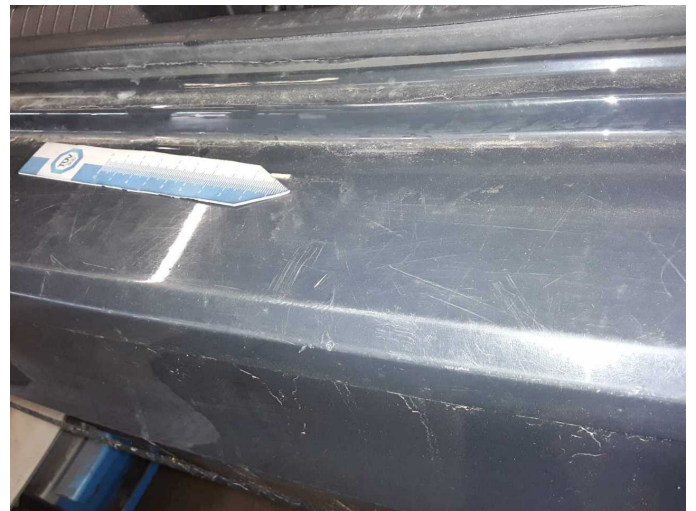
Damage 6: Rear bumper: Rear bumper - Scratch(es) - Paint
