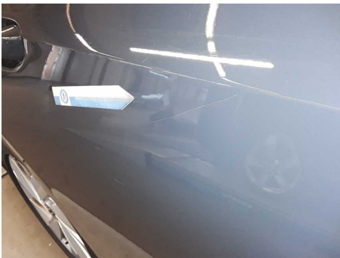
Damage 4: Door - rear right side: Door - Scratch(es) - Paint
