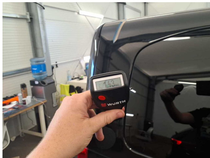
Repainting 1: Side panel - rear right side
