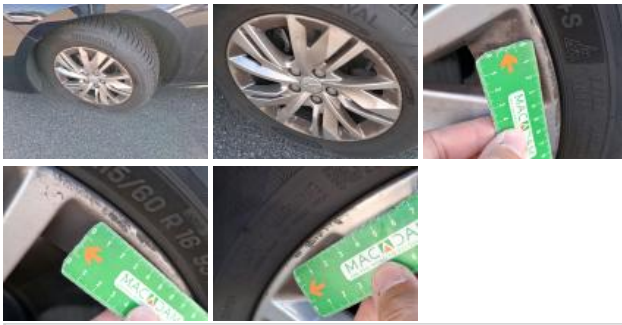
Alloy rim RL, Scratch(es), Acceptable
