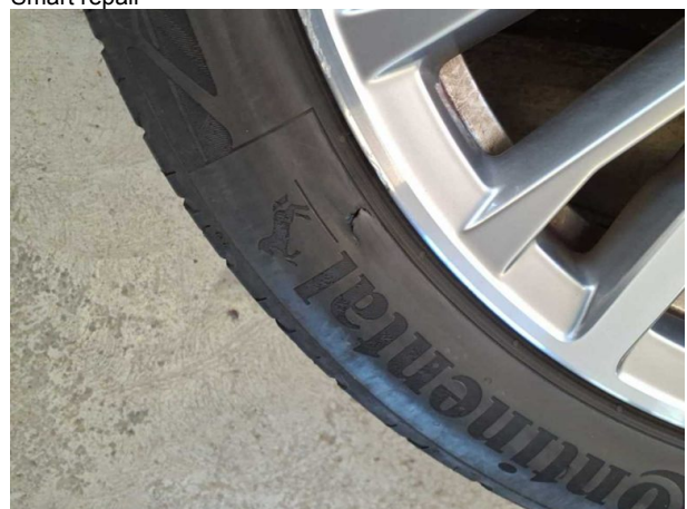
Damage #6: 2nd wheel set: 1 tyre - Damaged - Replace
