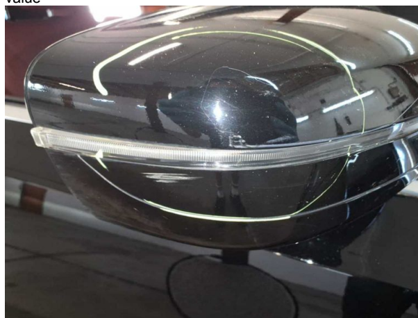
Damage #4: Wing mirror - right side: Cap - Scratched - Smart repair
