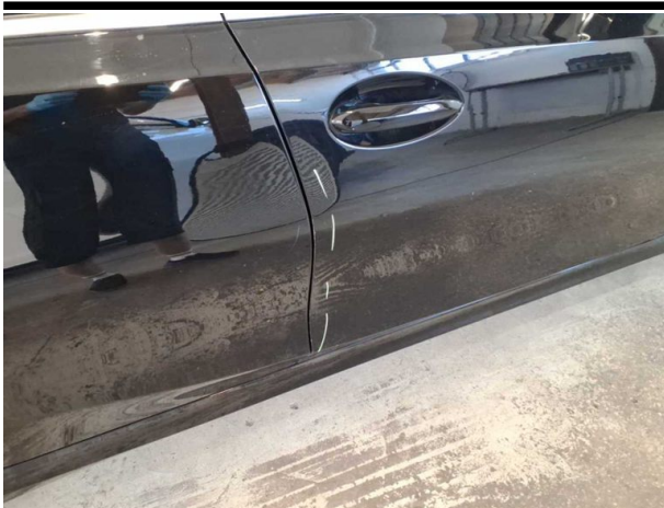
Damage #5: Door - front right side: Door edge - Scratched - Smart repair
