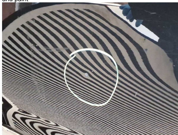
Damage #9: Door - rear left side: Door - Dent / paintcoat damage - Repair and paint
