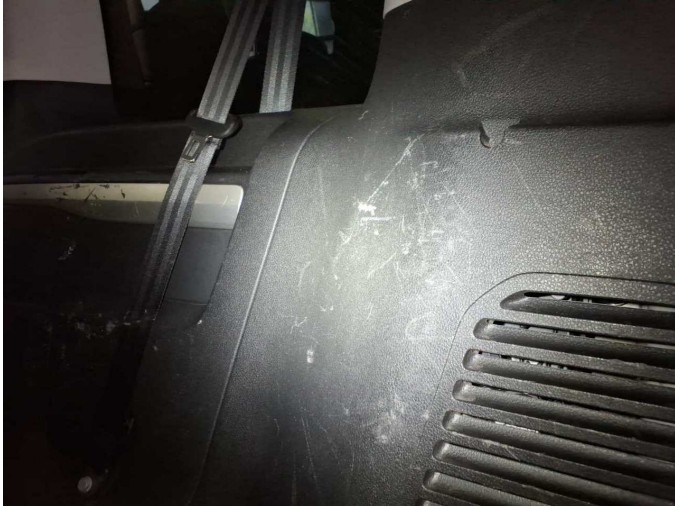
Damage 21: Side panel - rear right side: Interior trim - Scratched - Replace
