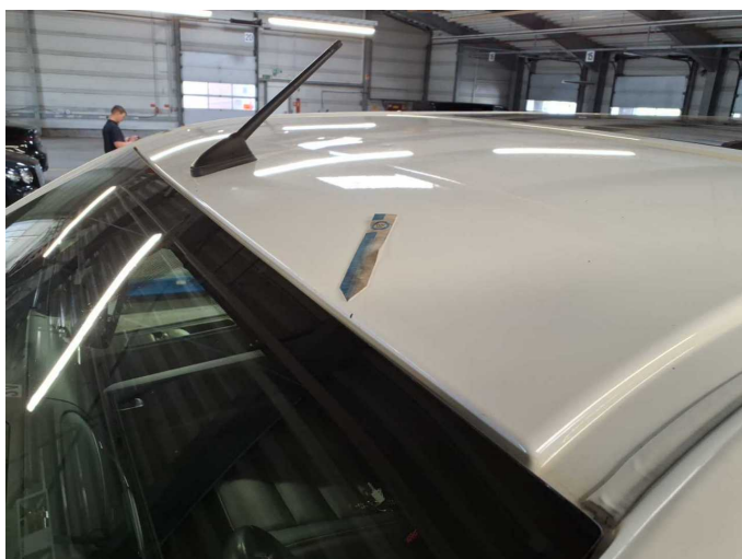
Damage 19: Roof: Roof - Dent / paintcoat damage - Paint
