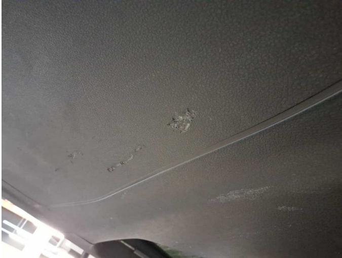
Damage 6: Trim / covers: Boot lid - interior trim - Scratch(es) - Loss in value
