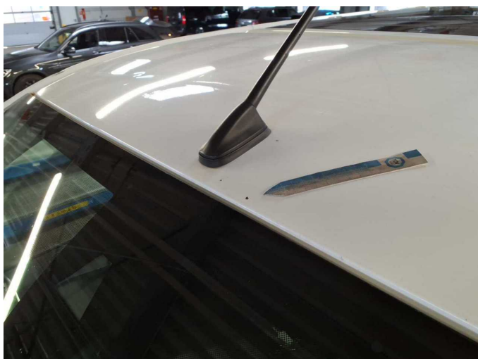
Damage 19: Roof: Roof - Dent / paintcoat damage - Paint
