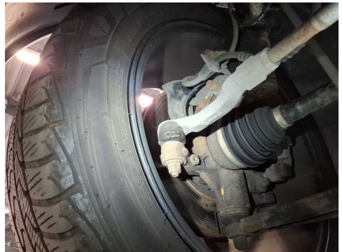
Damage 14: Steering system: Tie rod end (Links--> Achsvermessung) - Broken / torn - Replace
