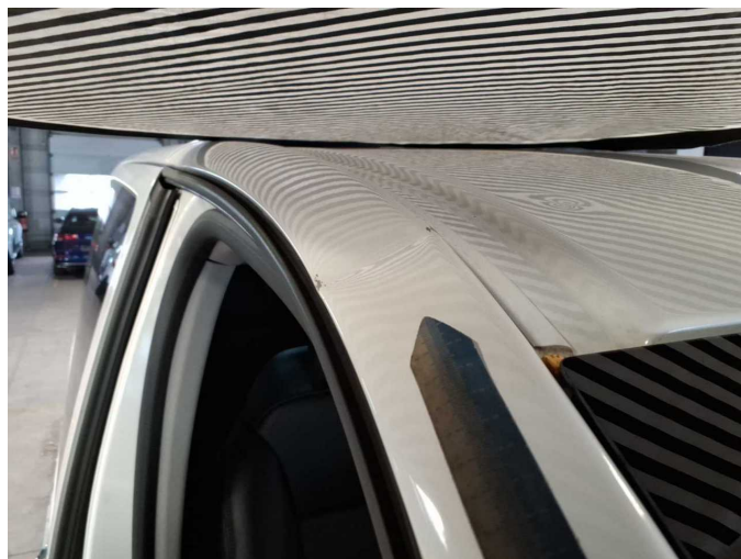
Damage 20: Body: A-pillar - right side - Deformed - Paint
