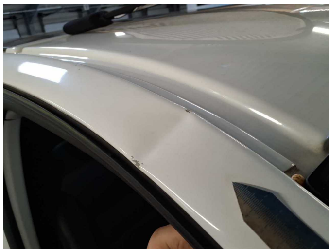
Damage 20: Body: A-pillar - right side - Deformed - Paint
