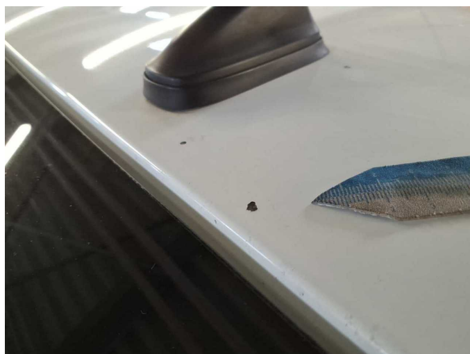
Damage 19: Roof: Roof - Dent / paintcoat damage - Paint
