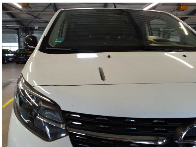
Damage 18: Bonnet: Bonnet - Stone chips - Paint
