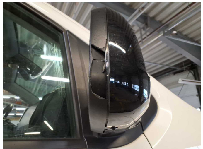
Damage 16: Wing mirror - right side: Mirror housing (Rahmen) - Broken / torn - Replace
