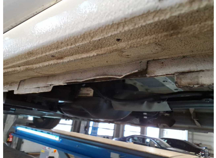
Damage 13: Sill - left side: Sill - Deformed - Smart repair
