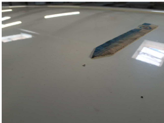
Damage 19: Roof: Roof - Dent / paintcoat damage - Paint
