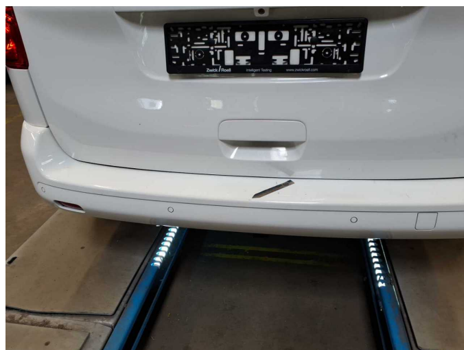
Damage 17: Rear bumper: Rear bumper - Scratched - Paint
