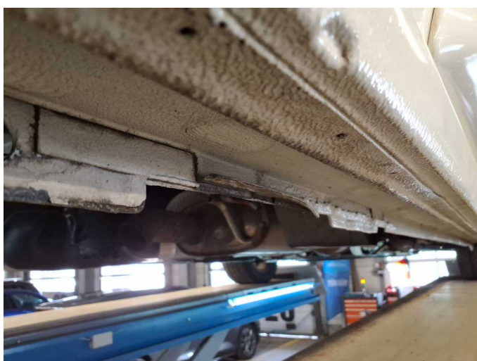
Damage 12: Sill - right side: Sill - Deformed - Smart repair
