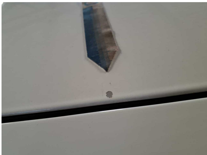
Damage 18: Bonnet: Bonnet - Stone chips - Paint
