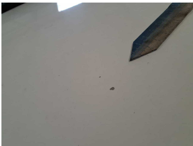
Damage 18: Bonnet: Bonnet - Stone chips - Paint
