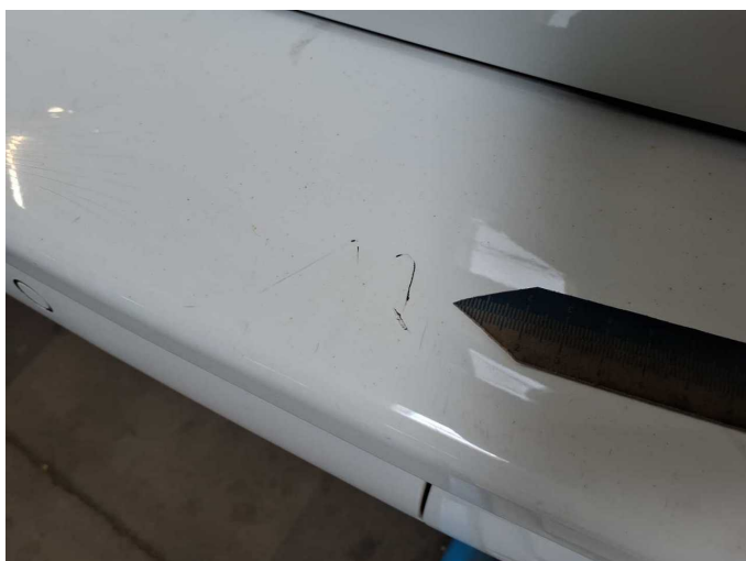
Damage 17: Rear bumper: Rear bumper - Scratched - Paint
