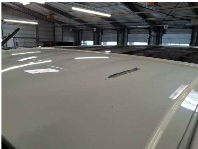
Damage 19: Roof: Roof - Dent / paintcoat damage - Paint
