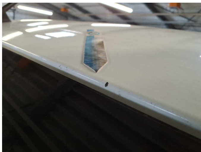
Damage 19: Roof: Roof - Dent / paintcoat damage - Paint
