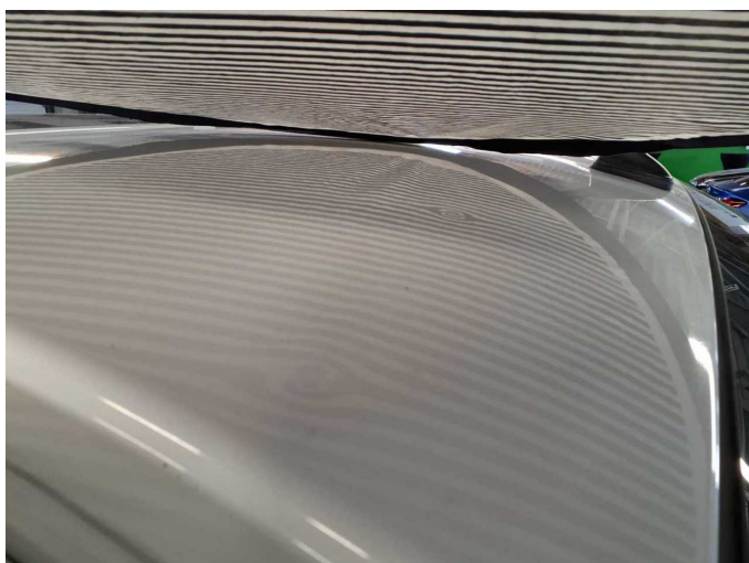
Damage 19: Roof: Roof - Dent / paintcoat damage - Paint
