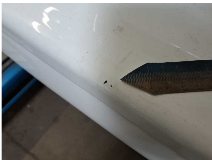
Damage 17: Rear bumper: Rear bumper - Scratched - Paint
