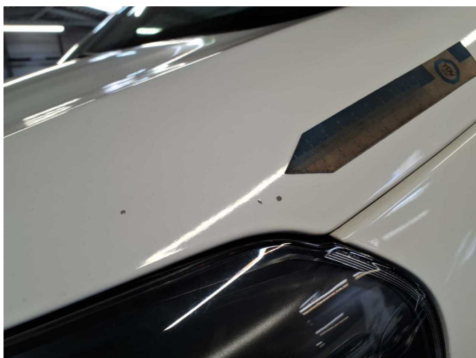
Damage 18: Bonnet: Bonnet - Stone chips - Paint
