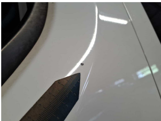
Damage 3: Door - front left side: Door - Stone chips - Smart repair
