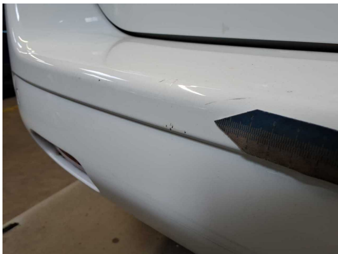
Damage 17: Rear bumper: Rear bumper - Scratched - Paint
