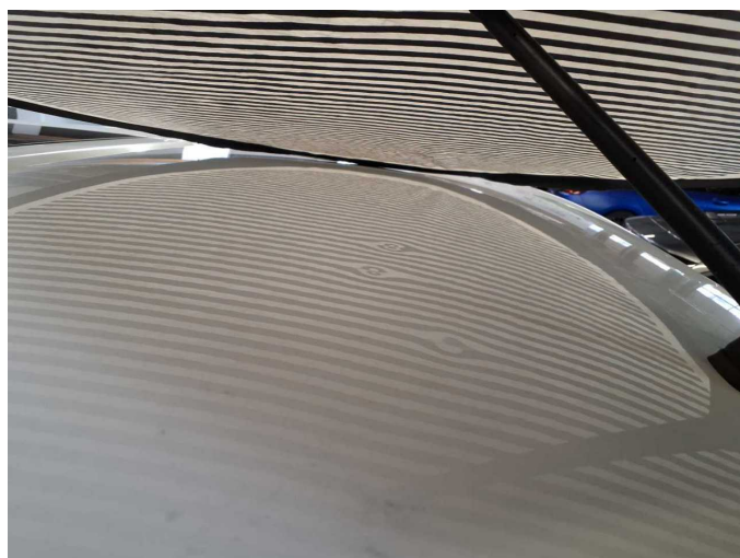
Damage 19: Roof: Roof - Dent / paintcoat damage - Paint
