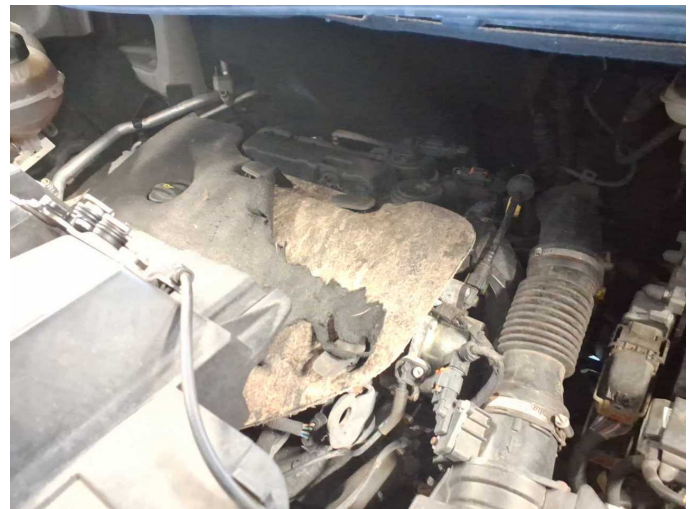
Damage 7: Engine: Engine cover - Broken / torn - Replace
