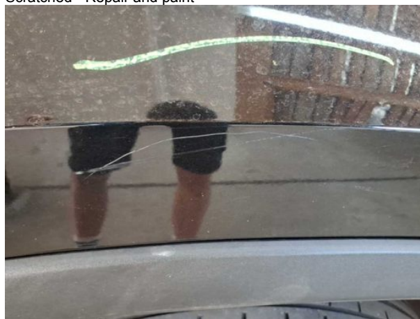
Damage #8: Mudguard - right side: Mudguard - right side - Scratched - Repair and paint
