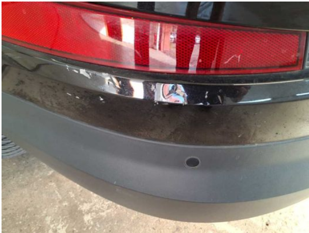
Damage #14: Rear bumper: Rear bumper - Damaged - Replace
