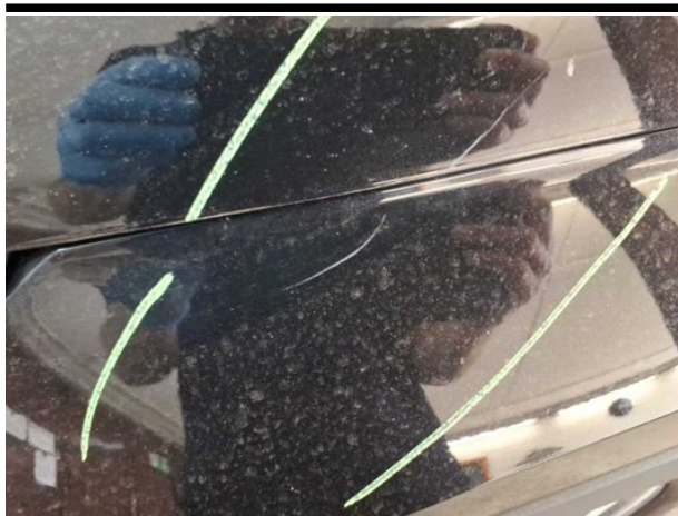
Damage #7: Mudguard - left side: Mudguard - left side - Scratched - Repair and paint
