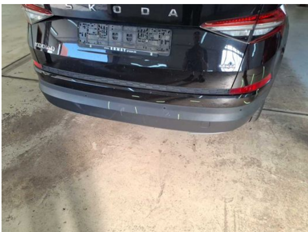
Damage #14: Rear bumper: Rear bumper - Damaged - Replace
