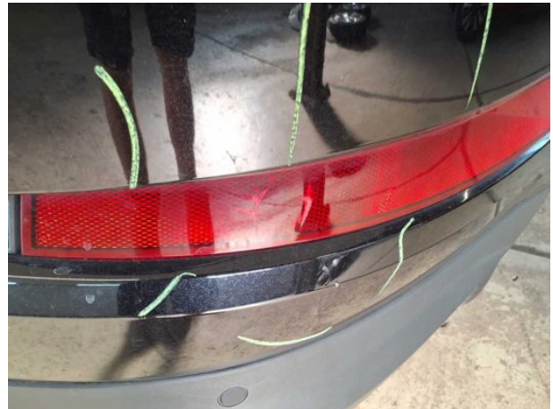
Damage #6: Boot lid / rear door: Reflectors - Damaged - Replace
