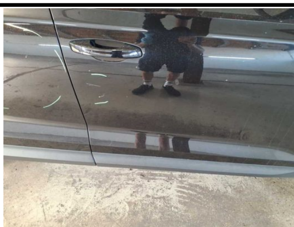
Damage #10: Door - front right side: Door - Scratched - Repair and paint
