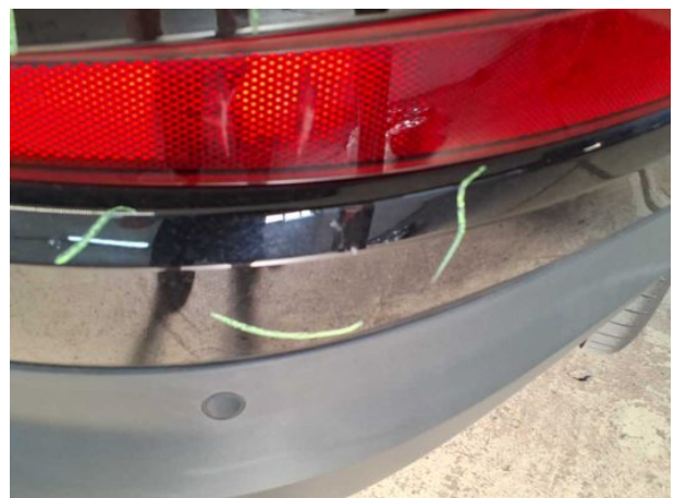
Damage #14: Rear bumper: Rear bumper - Damaged - Replace
