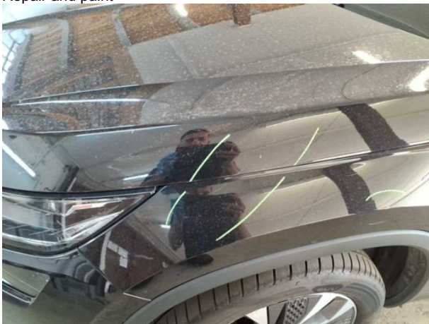
Damage #13: Bonnet: Bonnet - Scratched - Repair and paint
