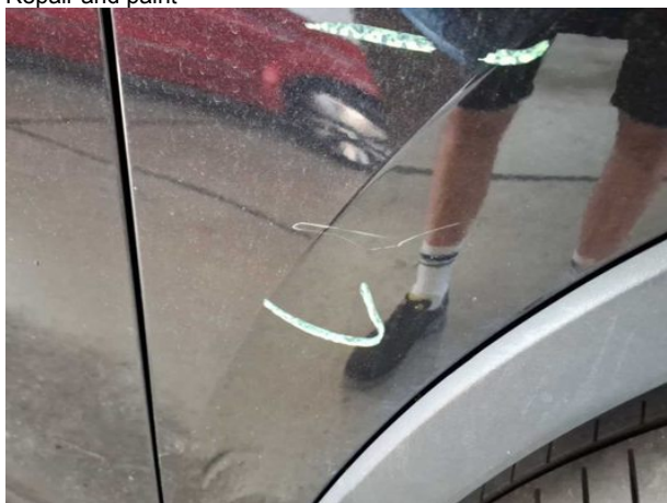
Damage #8: Mudguard - right side: Mudguard - right side - Scratched - Repair and paint
