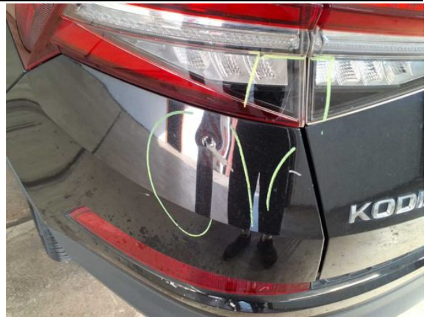
Damage #14: Rear bumper: Rear bumper - Damaged - Replace
