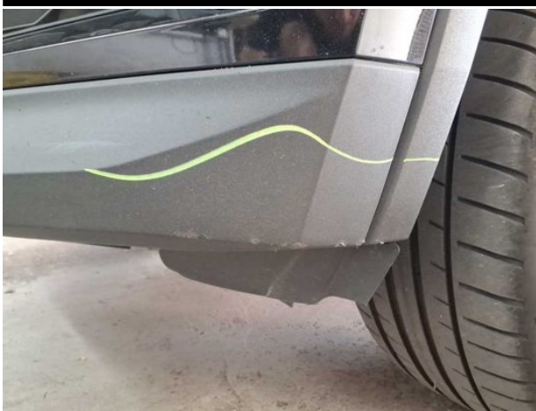
Damage #4: Front bumper: Spoiler - Scratched - Loss in value
