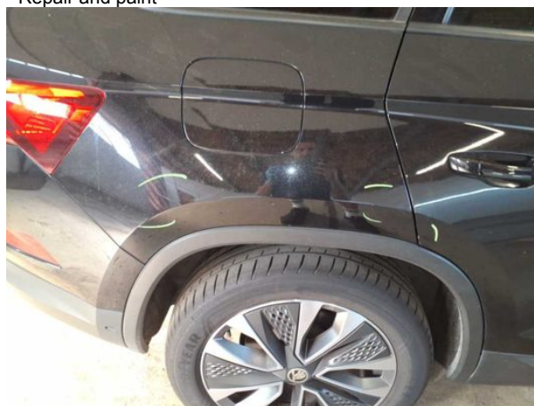
Damage #12: Side panel - rear right side: Side panel - Scratched - Repair and paint
