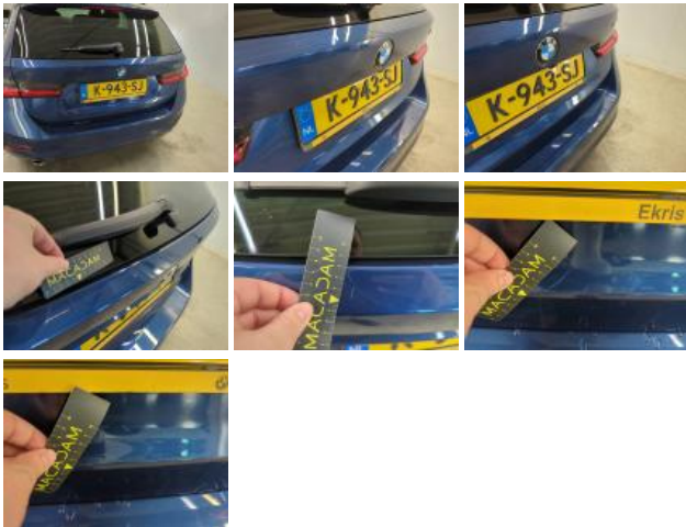
Bumper R, Scratch(es), Repair and paint (complete)
