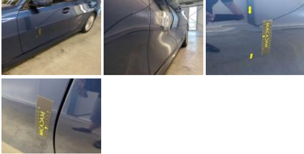
Outer sill L, Scratch(es), Repair and paint (complete)
