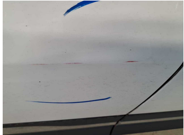
Damage #2: Door - rear right side: Door - Abrasion - Cover / polish
