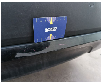
Bumper Rear // Repair & Painting-scratch + dent
