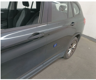
Door Rear Left // Repair & Painting-scratch + dent
