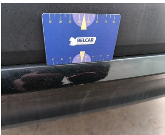
Bumper Rear // Repair & Painting-scratch + dent
