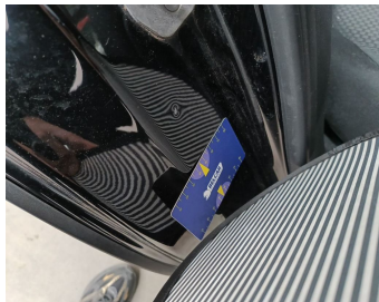
Rocker Panel Right // Smart Repair Medium-scratch + dent
