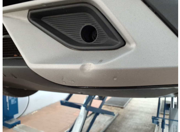
Damage 4: Front bumper: Front bumper (Blende) - Deformed - Replace
