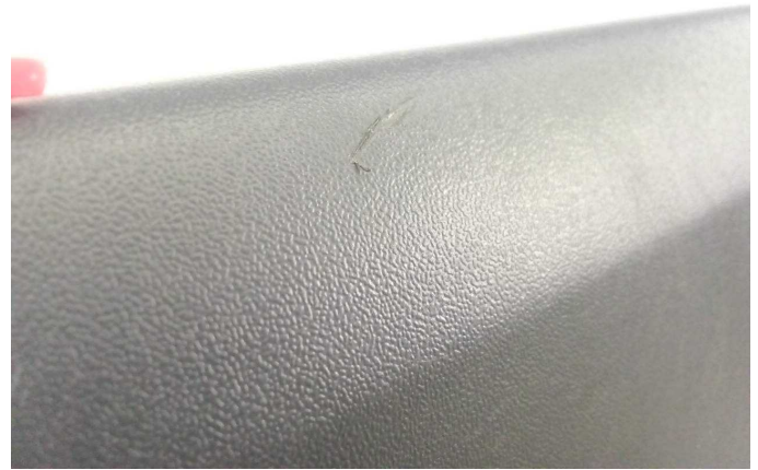
Damage 3: Rear bumper: Rear bumper - Scratched - Smart repair
