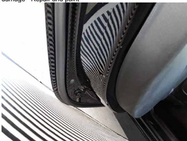
Damage #5: Door - rear left side: Door (Innen) - Dent / paintcoat damage - Repair and paint
