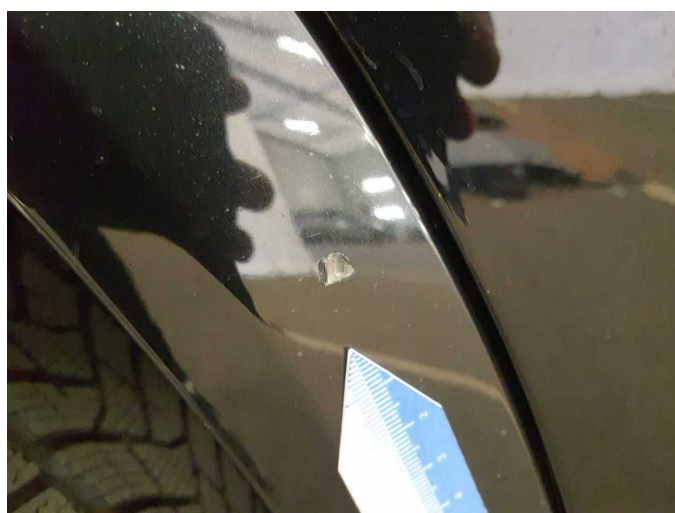
Damage 4: Side panel - rear right side: Wheel well extension - Stone chips - Smart repair
