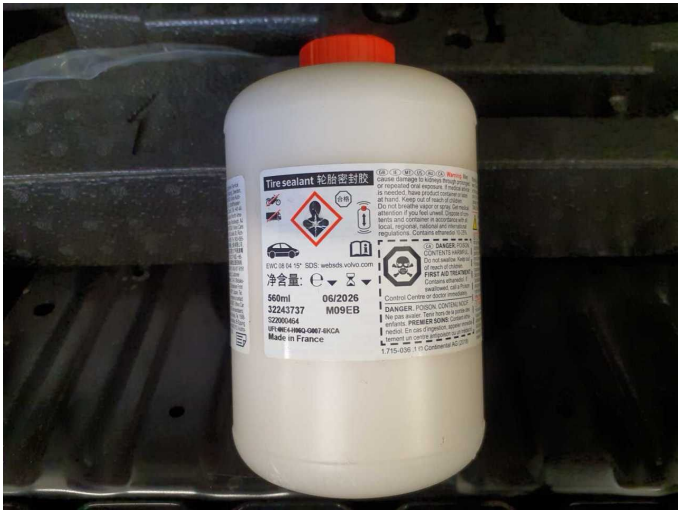
Damage 1: Equipment: Tirefit filler - Expired - Replace
