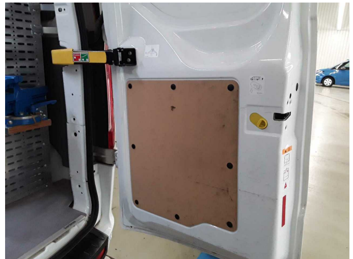
Damage 6: Boot lid / rear door: Trim rear door - plywood - lower (rechts) - Broken / torn - Replace
