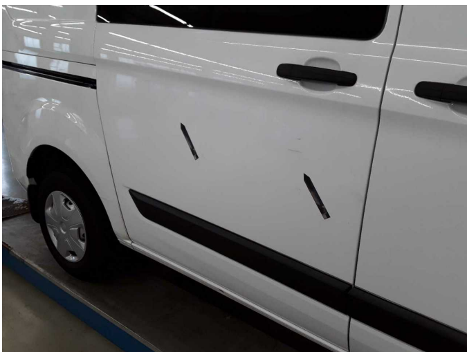
Damage 9: Sliding door, right: Sliding door with glass panel - Dent / paintcoat damage - Repair and paint
