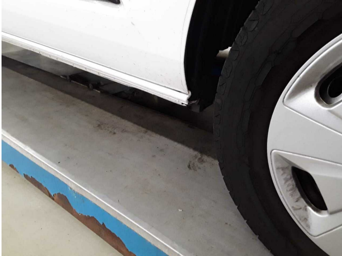
Damage 4: Mudguard - right side: Mud flap - Missing - Replace
