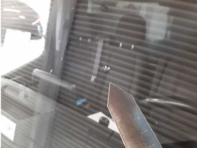
Damage 19: Vehicle glazing: Windscreen - Stone chips - Replace
