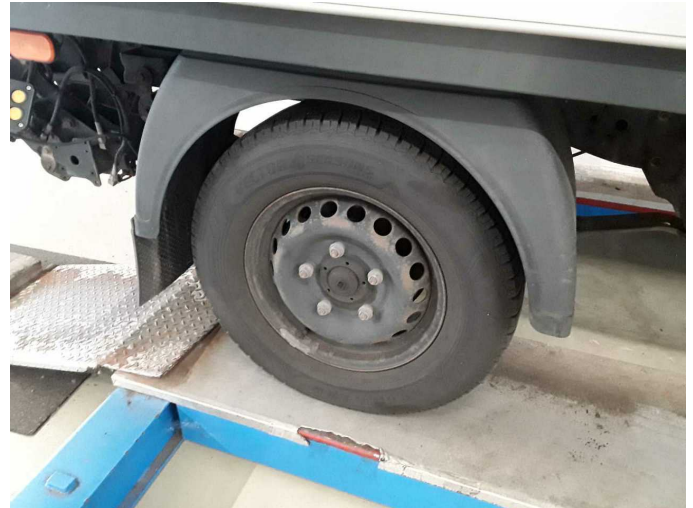
Damage 3: Wheel / tyres: Wheel cover - rear right side - Missing - Replace
