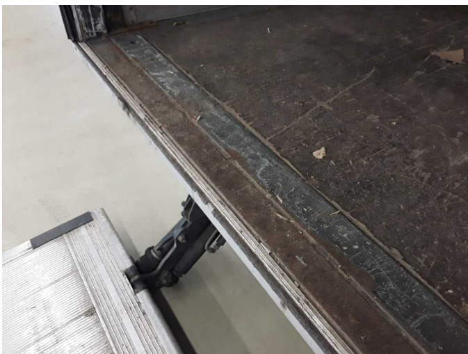
Damage 12: Misc.: Misc. (Planen-/Kofferaufbau) - Corrosion - Loss in value
