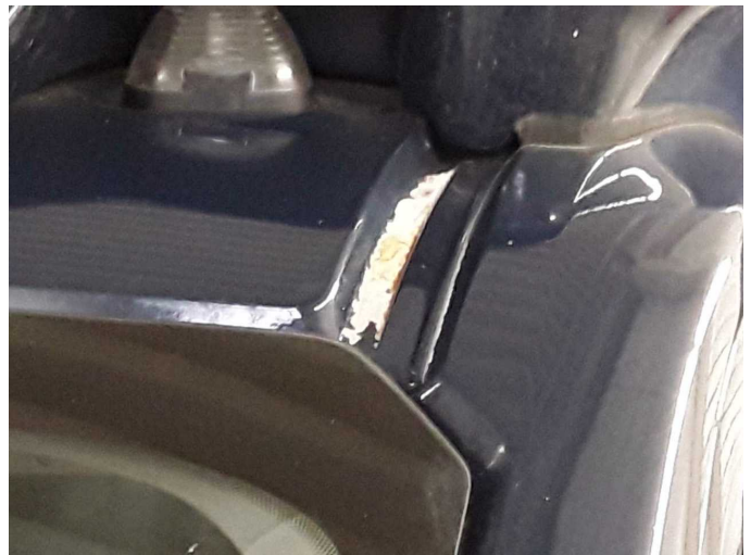
Damage 18: Roof: Roof - Paint defect - Paint
