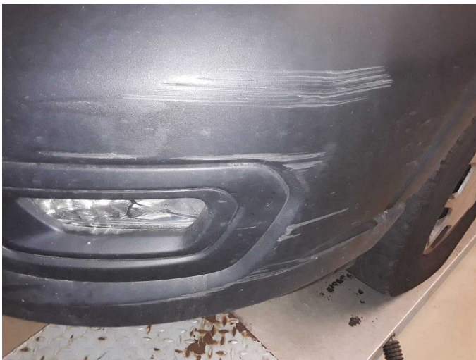
Damage 15: Front bumper: Front bumper (Unterteil) - Scratched - Replace
