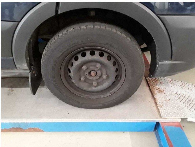
Damage 4: Wheel / tyres: Wheel cover - front right side - Missing - Replace
