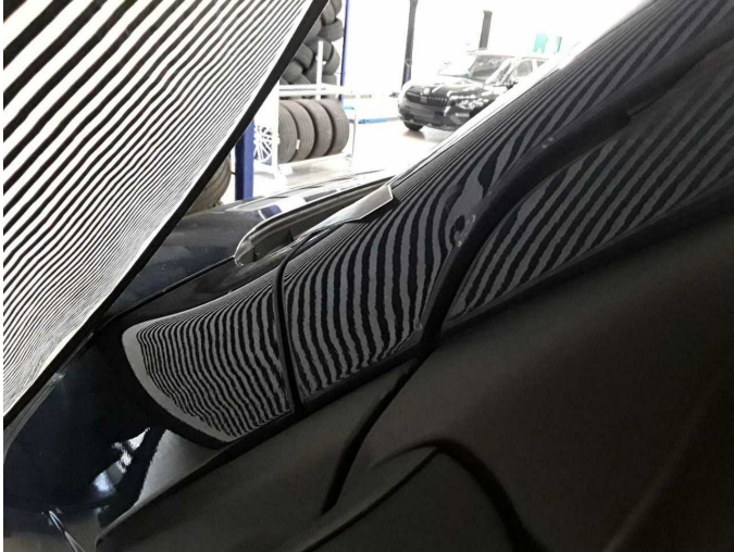
Damage 14: Body: A-pillar - left side - Dent / paintcoat damage - Repair and paint
