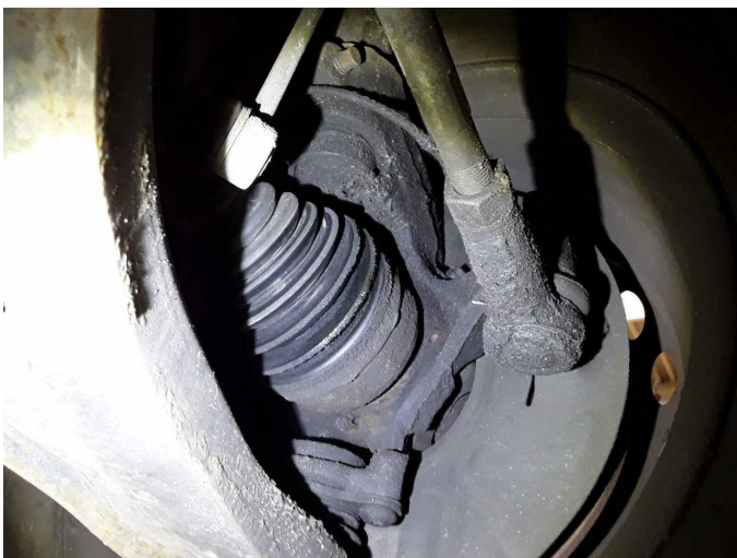
Damage 16: Drive train: Sleeve prop shaft - front right side - Leaking - Replace
