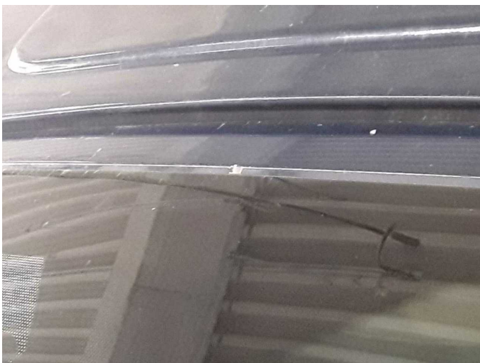
Damage 18: Roof: Roof - Paint defect - Paint
