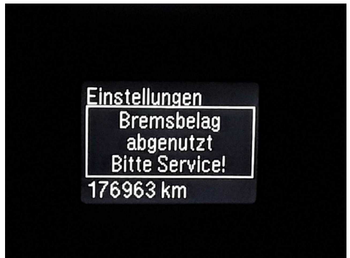
Damage 17: Braking system: Brake discs and brake pads - front - Worn - Replace
