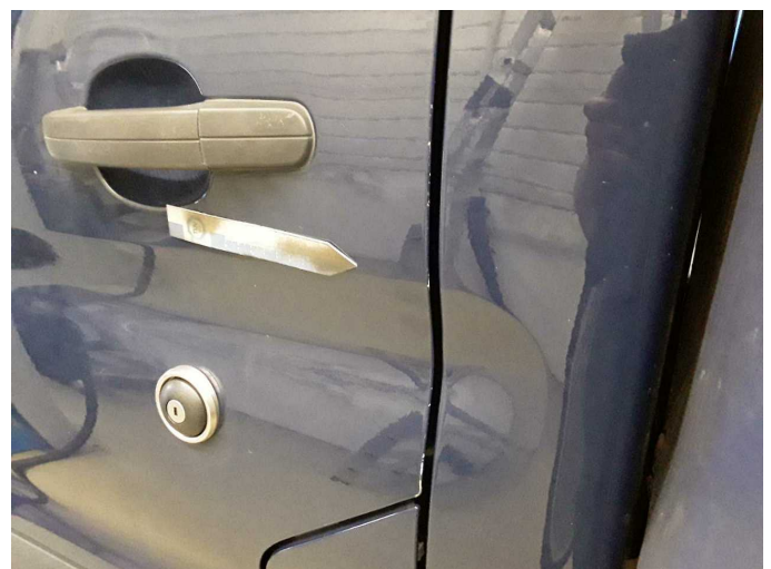
Damage 6: Door - front left side: Door edge - Scratch(es) - Smart repair
