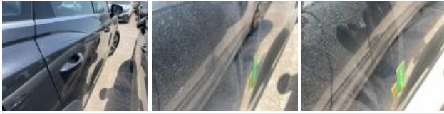
Bumper moulding R, Deformed / Strained, Replace
