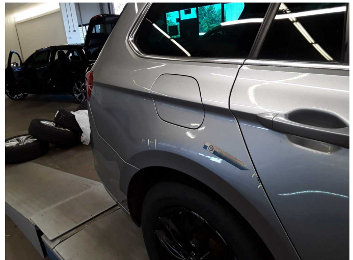
Damage 10: Side panel - rear right side: Side panel (Farbe) - Scratch(es) - Paint
