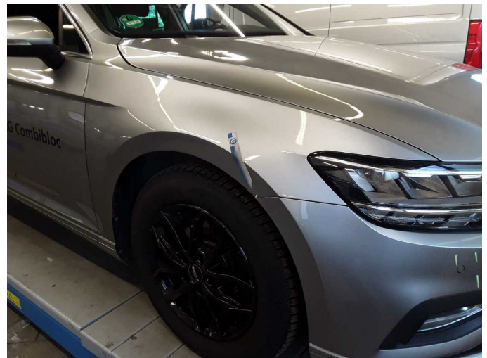
Damage 4: Mudguard - right side: Mudguard - right side (Farbe) - Paint defect - Smart repair
