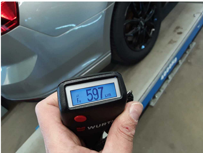
Repainting 1: Mudguard - right side, Bonnet, Side panel - rear right side, Door - front left side
