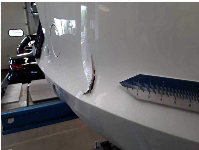
Damage 4: Rear bumper: Rear bumper - Broken / torn - Replace
