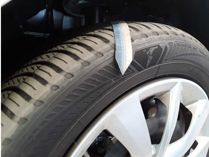
Damage 3: Wheel / tyres: Tyre - front (Beide) - Does not meet the leasing specifications - Replace
