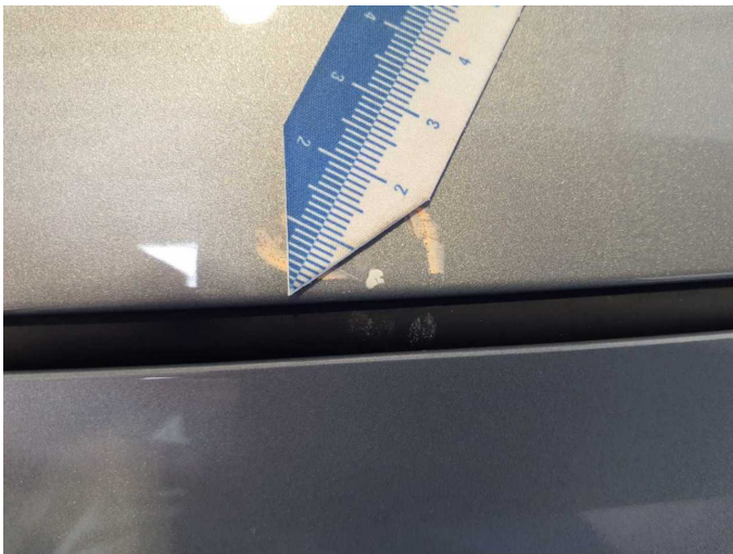
Damage 6: Bonnet: Bonnet - Stone chips - Paint
