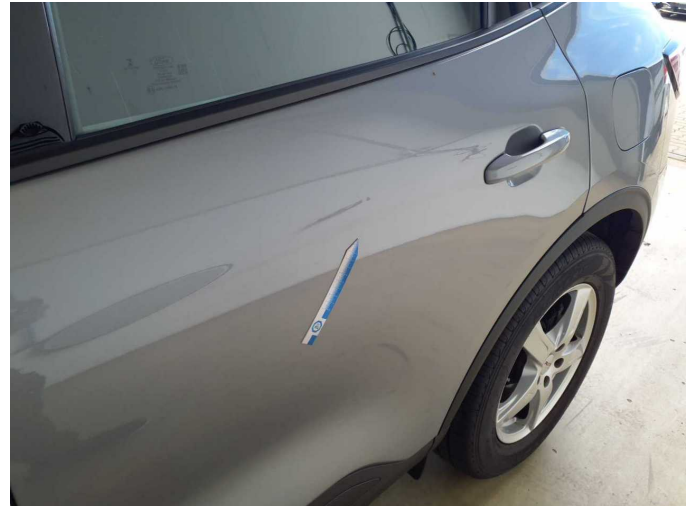
Damage 3: Door - rear left side: Door - dent(s) - Smooth repair work
