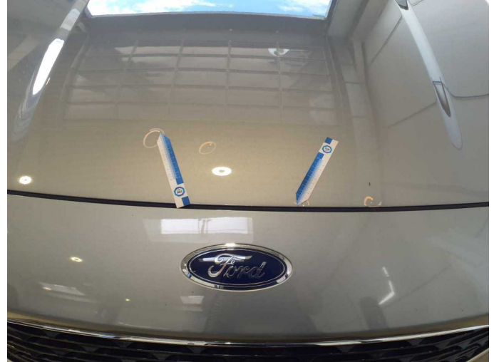
Damage 6: Bonnet: Bonnet - Stone chips - Paint
