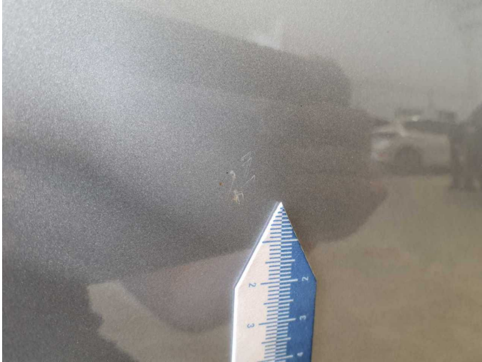
Damage 5: Door - front right side: Door - Scratch(es) - Paint
