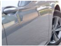
Door FR, Dent(s), Paintless dent repair
