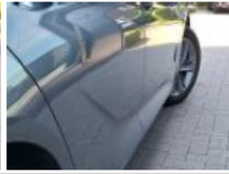
Door FR, Dent(s), Paintless dent repair
